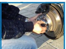
Mount the wheel spacer on the axle using the nuts/bolts which were included in the delivery. Tighten the nuts/bolts by hand.
