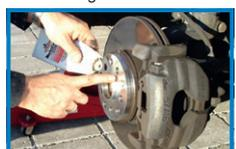
Place the wheel spacer on the vehicle hub and then also apply a thin layer of corrosion protection paste to the centering flange on the spacer.
