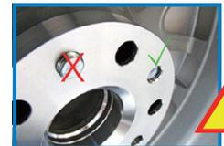
System 4 - 13xxx Please check that the bolts you are using to fix wheel to spacer when tight are at least 2mm shorter than thickness of spacer.
