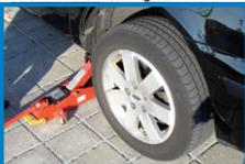
Lift the vehicle until the tire is off the ground, then place an axle stand under the vehicle.
