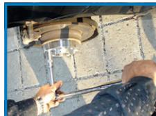
Using a torque wrench. Tighten crossways to the vehicle manufacturers specifications. Check twice.
