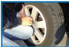
Locate the wheel, fix with bolts and hand tighten.
