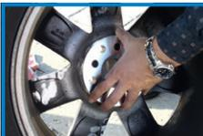
Check that the spacer is completely in contact with the mounting surface of the wheel.
