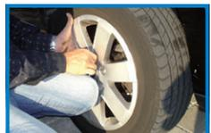
Locate the wheel, fix with the new nuts/bolts and tighten by hand.
