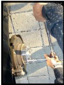
Using a torque wrench. Tighten crossways to the vehicle manufacturers' specifications. Check twice.
