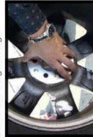
**9** Auch an der Achse muss die Distanzscheibe vollflächig anliegen. Check that the spacer is in complete contact with the vehicle hub, mounting surface and that the depth of the flange is not fouling the spacers flange.
