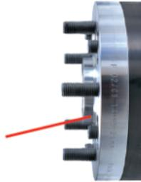
*System 3 - 14xxx You must consider that the original vehicle studs can protrude the mounting surface of the new spacer (15, 20, 25 and 30mm). If the wheel has no relief pockets then the vehicle studs will need to be shortened to allow the wheel to sit flat to the mounting face of the spacer. This will always apply to System 3 15mm.*
