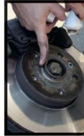
*Apply a thin layer of corrosion protection paste to the centering flange on the spacer.*
