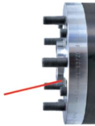
*System 3 - 14xxx You must consider that the original vehicle studs can protrude the mounting surface of the new spacer (15, 20, 25 and 30mm). If the wheel has no relief pockets then the vehicle studs will need to be shortened to allow the wheel to sit flat to the mounting face of the spacer. This will always apply to System 3 15mm.*
