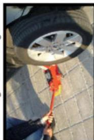
Raise the vehicle enough to remove the axle stands, then slowly lower the lifting jack.
