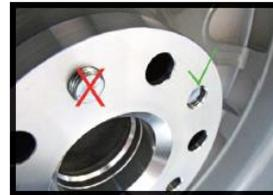
*System 4 - 13xxx Please check that the bolts you are using to fix wheel to spacer when tight are at least 2mm shorter than thickness of spacer.*
