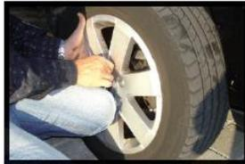
*Locate the wheel, fix with the new nuts/bolts and tighten by hand.*
