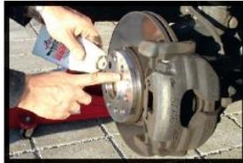
*Place the wheel spacer on the vehicle hub and then also apply a thin layer of corrosion protection paste to the centering flange on the spacer.*
