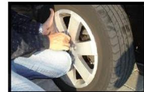
*Locate the wheel, fix with bolts and hand tighten.*
