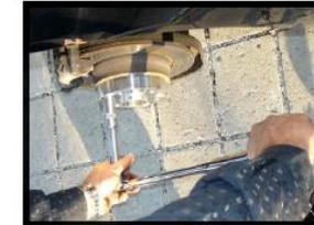
*Using a torque wrench. Tighten crossways to the vehicle manufacturers specifications. Check twice.*
