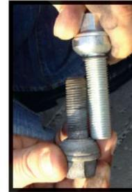
Check if the length and type of seating of the new and longer bolts are correct. (Have a look overleaf at the bolts advice. The new fixings need to be as long as the originals plus the thickness of the spacer.
