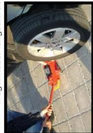
Raise the vehicle enough to remove the lower the lifting jack.
