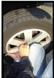
Locate the wheel, fix with the new nuts/bolts and tighten by hand.
