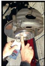
Place the wheel spacer on the vehicle hub and then also apply a thin layer of corrosion protection paste to the centering flange on the spacer.
