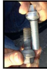
Check if the length and type of seating of the new and longer bolts are correct. (Have a look overleaf at the bolts advice. The new fixings need to be as long as the originals plus the thickness of the spacer.
