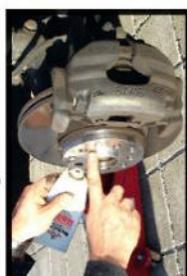
Place the wheel spacer on the vehicle hub and then also apply a thin layer of corrosion protection paste to the centering flange on the spacer.
