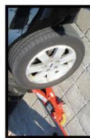
*Lift the vehicle until the tire is off the ground, then place an axle stand under the vehicle.*
