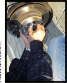
Mount the wheel spacer on the axle using the nuts/bolts which were included in the delivery. Tighten the nuts/bolts by hand.
