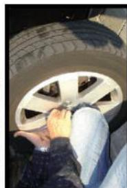
Locate the wheel, fix with the new nuts/bolts and tighten by hand.
