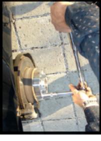
Using a torque wrench. Tighten crossways to the vehicle manufacturers' specifications. Check twice.
