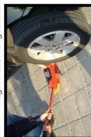
Raise the vehicle enough to remove the jacks, then slowly lower the lifting jack.
