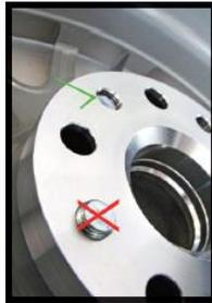
System 4 - 13xxx Please check that the bolts you are using to fix wheel to spacer when tight are at least 2mm shorter than thickness of spacer.
