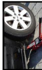
*Position the lifting jack and take the pressure off the wheel.*
