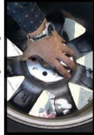
**9** Auch an der Achse muss die Distanzscheibe vollflächig anliegen. Check that the spacer is in complete contact with the vehicle hub mounting surface and that the depth of the flange is not fouling the spacers flange.
