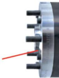
System 3 - 14xxx You must consider that the original vehicle studs can protrude the mounting surface of the new spacer (15, 20, 25 and 30mm). If the wheel has no reiler pockets then the vehicle studs will need to be shortened to allow the wheel to sit flat to the mounting face of the spacer. This will always apply to System 3 15mm.
