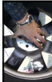
*Check that the spacer is completely in contact with the mounting surface of the wheel.*
